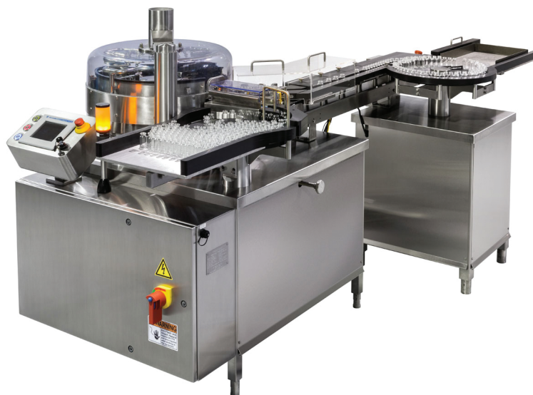
FIGURE 3. The PennTech RW-500 rotary vial washer. Photograph courtesy of PennTech Machinery Corporation, Warminster, Pennsylvania, USA.
