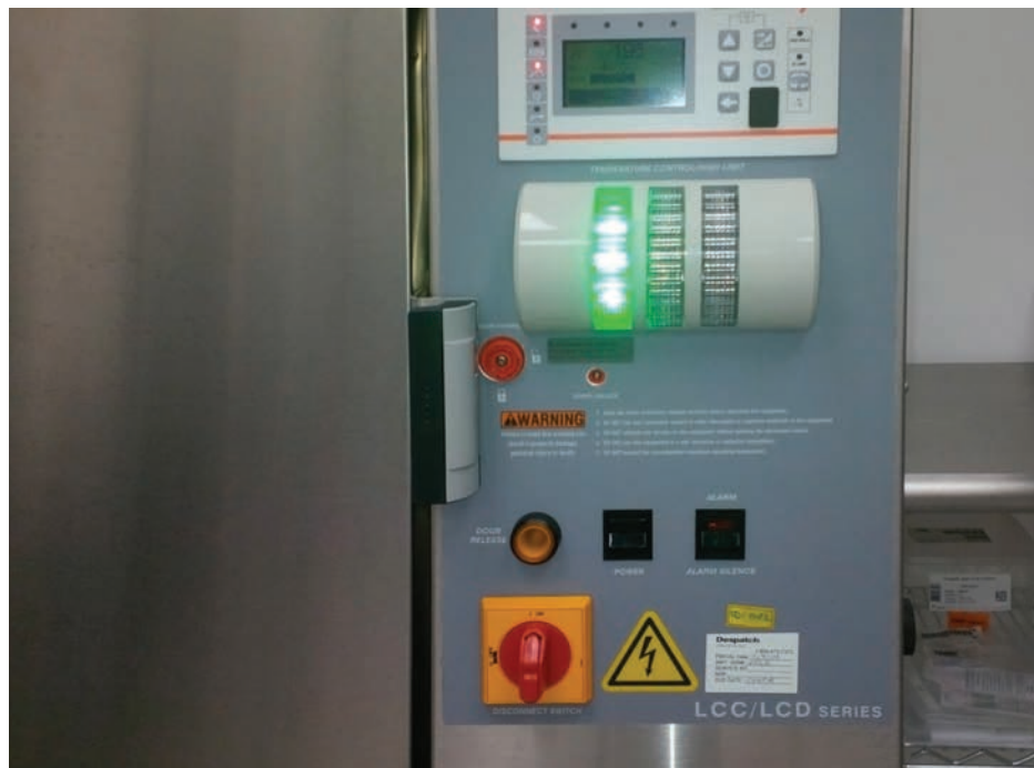
FIGURE 3. A three-color light on the Despatch LCC1-51-4 oven (Despatch Industries, Lakeville, Minnesota) shows the status of the depyrogenation process. A green light (above) indicates the cycle in progress; an amber light, an idling oven; and a red light, a high-temperature limit.
